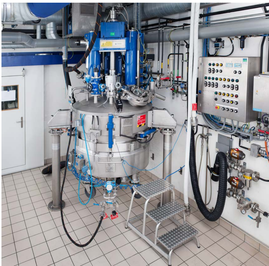
Fig. 2b. Large-scale reactor for SPPS allowing to produce kilograms of peptide.
